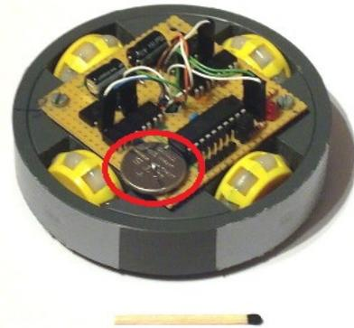
Figure 1. An image of a disassembled Haptic Prop. Notice the single CR2032 battery, which can power the device for up to 5000h.
